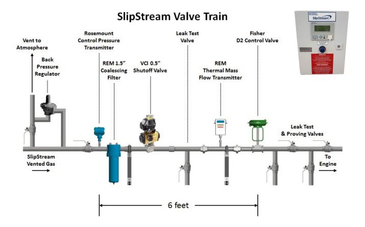
This newly developed addition to the SlipStream<sup>®</sup> family is designed to work with any OEM, REMVue or REAcct controlled engines.
